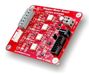
The heart of the board is Si9986, it is an integrated, buffered H-bridge with TTL compatible inputs and the capability of delivering a continuous 1.0Amp at 12 V with switching rates up to 200 kHz. By supporting high-frequency pulse width modulation (PWM), the DC motor can run smoothly and quietly over a wide speed range. This board includes two LED's to show the PWM input signal states. Heavy duty screw terminal
