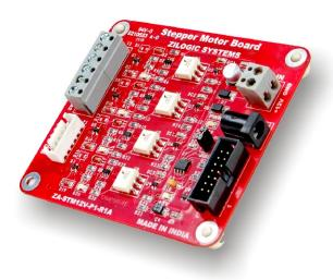
This board offers a high degree of isolation with the use of high speed opto-isolators for isolation between low voltage control side and high voltage motor drive side. It also comes with series of LEDs to indicate each phase of the stepper signals. Power-on delay circuit is provided to give sufficient time to MCU/Control logic to initialise the stepper input signals to known state thereby avoiding momentary glitches on the motor circuit.
