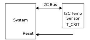
The temperature sensor can act like a thermal watchdog using the  $T\_CRIT$  signal. The  $T\_CRIT$  becomes low when the temperature exceeds the  $T\_CRIT$  setpoint. The  $T\_CRIT$  is held low till the temperature drops by a configurable hysteresis amount.
