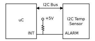
The temperature sensor has an **ALERT** signal that can be used as an interrupt signal. The set points for local and remote temperatures can be configured individually. An example circuit configuration is shown in Figure 2.3, "Alert Interrupt". Note that since the **ALERT** is an open collector output a pull-up resistor (typically 10k) is required. The pseudo code for enabling interrupt notification when the local temperature exceeds the range 10 °C - 60 °C is given below.
